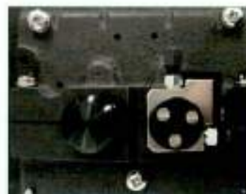
Dual-beam optical design with reference cell (left) and flow cell (right)
