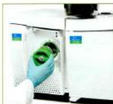
A simple twist and pull is all that is required to access the tool-free SMARTsource on the Clarus SQ 8 GC/MS.
